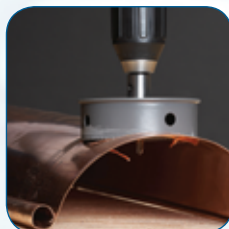
Outlet Saw cutting progression in half round gutter.
